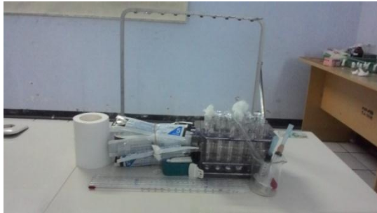
Peralatan praktikum LED: (rak tabung westergren, tabung westergren, spuit, tourniquet, pipet tetes, rak tabung reaksi, tabung reaksi, vial, beaker glass, botol kaca)
