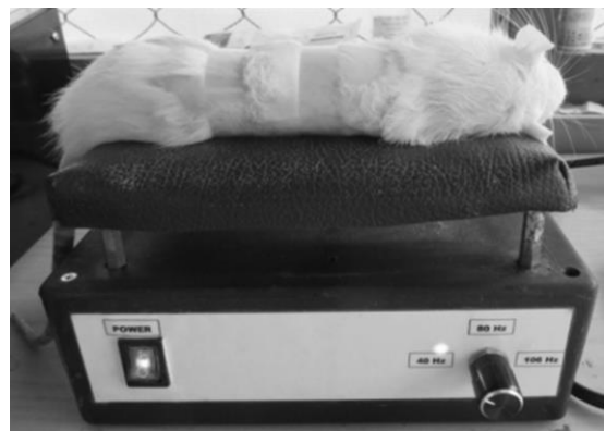
Figure 3. Rat was placed on the vibrating device. The wound is at the centre of the vibrating device.
